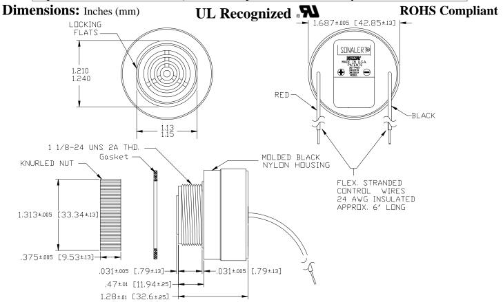
NOTE A: MOUNTING- REMOVE BLACK PLASTIC NUT WHILE LEAVING GASKET ON THREADED NECK OF ALARM. INSERT THREADED NECK THROUGH APPROPRIATE SIZED PANEL HOLE, SCREW NUT BACK ONTO THREADED FRONT
